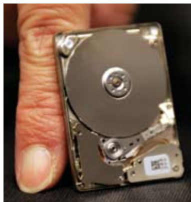
TINY HARD DRIVES are creating new industries. This one, introduced by Hitachi in January, can hold 10 gigabytes.
