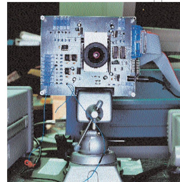
This artificial eye contains working electronic versions of the four types of ganglia cells in the retina. The cumbersome array of electronics and optics surrounds an artificial retina, which is just one-tenth of an inch wide.
